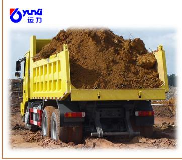
Make & Model : YUNLI MGW430 Operating Weight (GVW): 43,000 kg Bucket capacity: ±16 m3 Engine type: Diesel 6 inline cylinder – Euro II Direct fuel injection. Turbo-charge intercooler. Engine power: 336 hp / 247kw @2200 rpm. Power train: 6x4 c/w hub reduction. Transmission: Manual -10 forward & 2 reverse. Max speed: 78 km/hr. Gradeability: 50% (28 °)
